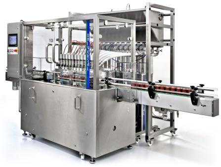
Posimatic EV Servo is a fully-automatic volumetric filling system which uses servo drives rather than pneumatic air cylinders.
